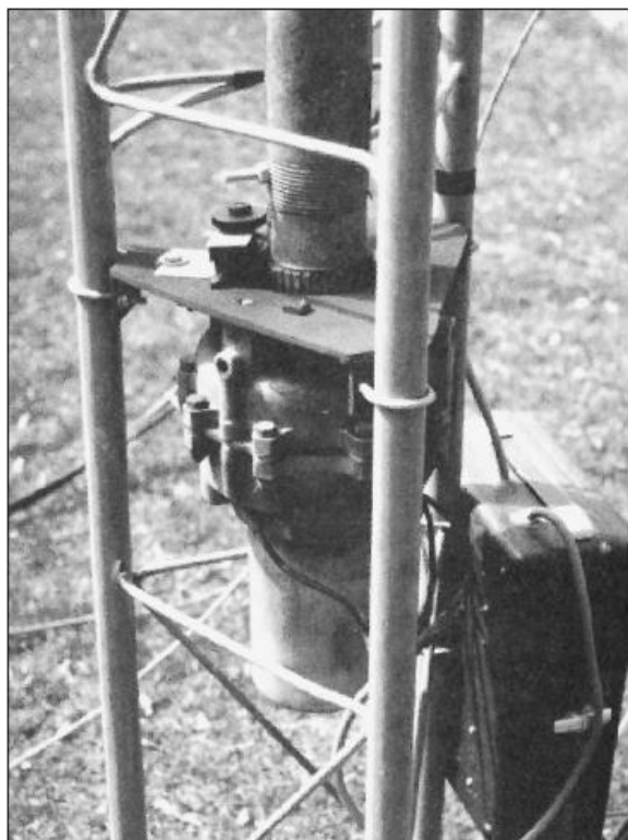
Figure 2 — Azimuth rotation systems, showing prop-pitch motor and position sensor.
